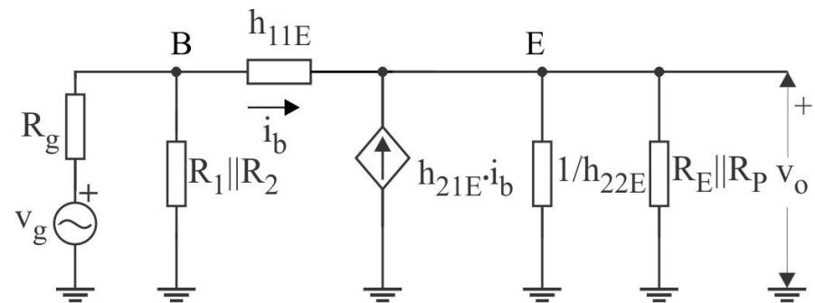
$$R_{EC} = R_E \parallel R_p$$
