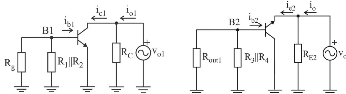
$$R_{out1} = \frac{v_{o1}}{i_{o1}}$$
