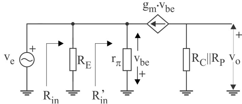
$$v_o = -g_m \cdot v_{be} \cdot R_C \parallel R_P$$
