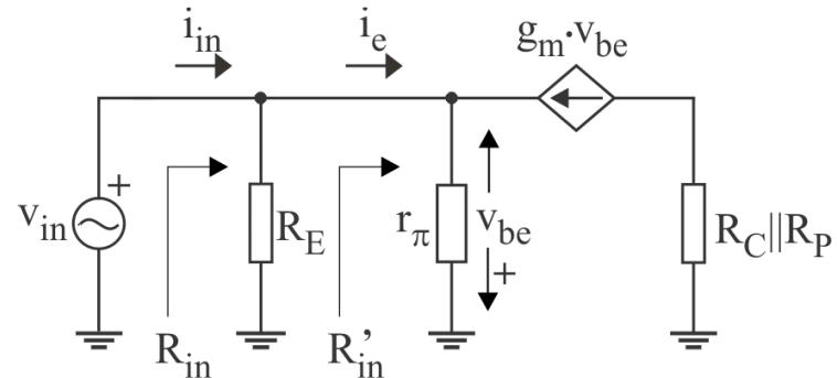
$$i_e = \frac{v_e}{r_\pi} - g_m \cdot v_{be} = v_e \cdot \left( \frac{1}{r_\pi} + g_m \right) = v_e \cdot \left( \frac{1}{r_\pi} + \frac{\beta}{r_\pi} \right)$$
