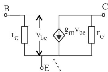
$$g_m = \frac{I_C}{V_T} \quad r_\pi = \frac{V_T}{I_B} \quad V_T = \frac{K \cdot T}{q} = 26 \text{ mV}$$
