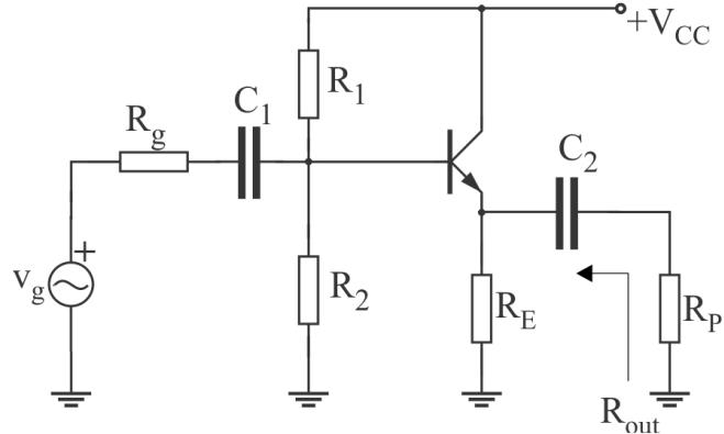
$$r_\pi = h_{11E} \quad h_{21E} = \beta \quad R_{BC} = R_1 || R_2 \parallel R_g$$
