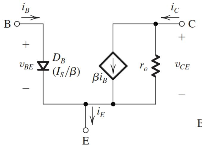
$$i_B = \left(\frac{I_S}{\beta}\right) e^{\frac{v_{BE}}{V_T}}$$
