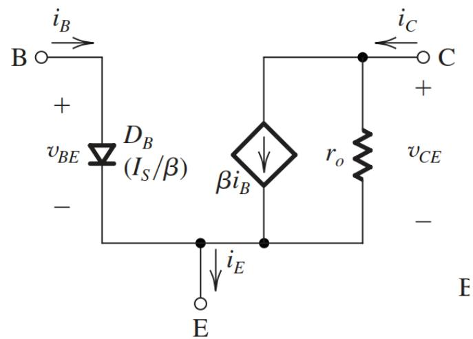
$$i_B = \left( \frac{I_S}{\beta} \right) e^{v_{BE}/V_T}$$
