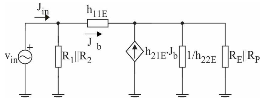
$$R_{EC} \ll \frac{1}{h_{22e}} \Rightarrow R_{EC} \parallel \frac{1}{h_{22e}} \approx R_{EC}$$
