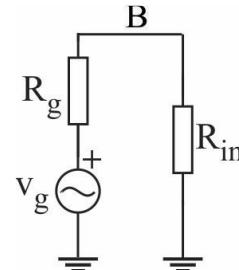
$$\frac{v_b}{v_g} = \frac{R_{in}}{R_g + R_{in}}$$
