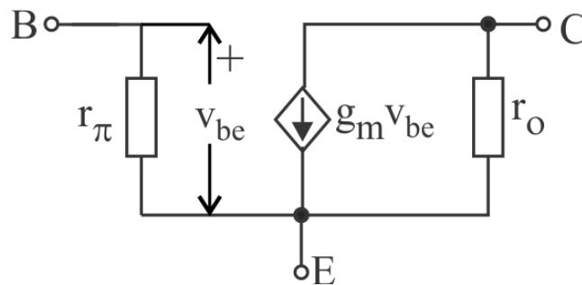
$$r_\pi = \frac{v_{BE}}{i_B} = \frac{V_T}{I_{BQ}}$$
