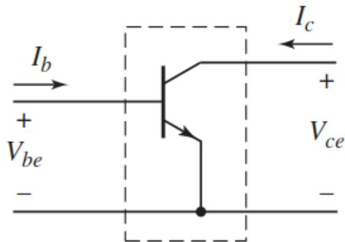
$$\Delta v_{BE} = \frac{\partial v_{BE}}{\partial i_B} \cdot \Delta i_B + \frac{\partial v_{BE}}{\partial v_{CE}} \cdot \Delta v_{CE}$$
