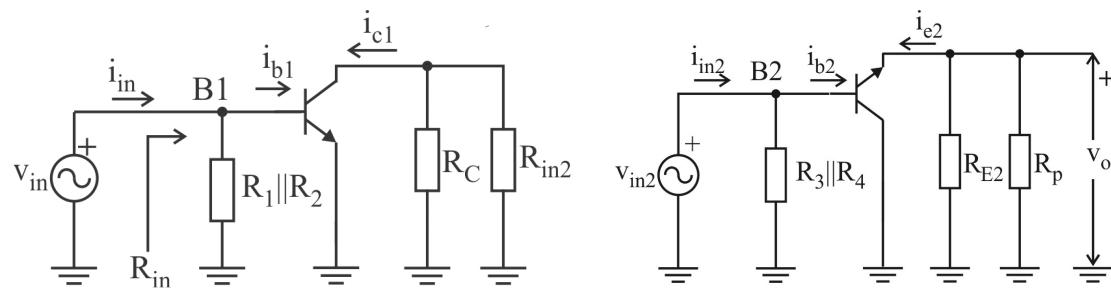
$$R_{in} = R_{in1} = \frac{v_{in}}{i_{in}}$$
