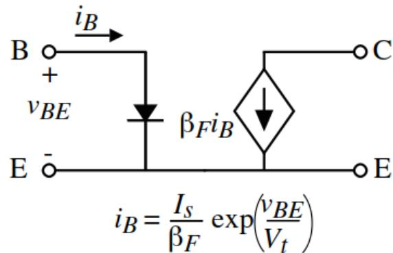
$$i_B = \frac{I_s}{\beta} \cdot \exp\left(\frac{v_{BE}}{V_T}\right)$$
