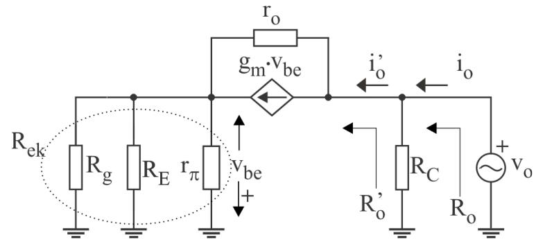
$$R_{ek} = R_g \parallel R_E \parallel r_\pi$$
