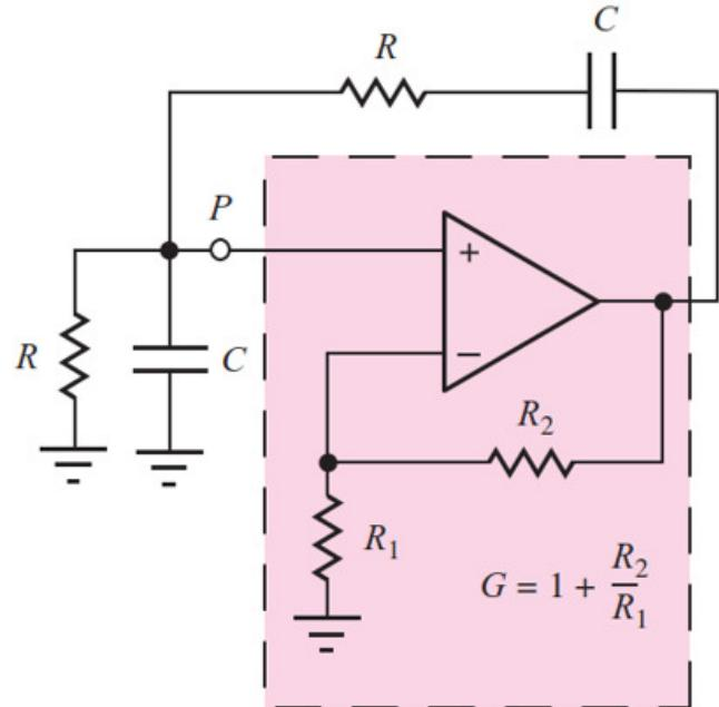
$$A \cdot B(j\omega) = \frac{1 + R_2/R_1}{3 + j(\omega CR - \frac{1}{\omega CR})}$$
