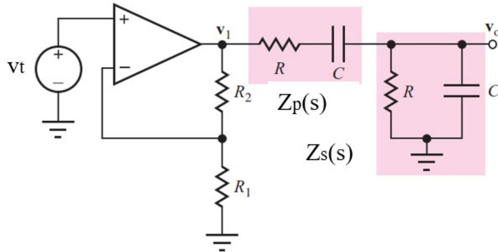
$$AB(j\omega) = \frac{v_o(j\omega)}{v_t(j\omega)} = \frac{1 + R_2/R_1}{3 + j(\omega CR - \frac{1}{\omega CR})}$$
