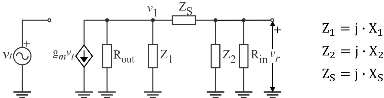
$$A \cdot B = \frac{v_r}{v_t} = \frac{v_1}{v_t} \cdot \frac{v_r}{v_1} = \frac{-g_m \cdot R_{out} \cdot Z_1 \cdot Z_2}{Z_1 \cdot (Z_2 + Z_S) + R_{out} \cdot (Z_2 + Z_S) + R_{out} \cdot Z_1}$$
