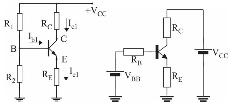
$$V_{BB} = \frac{R_2}{R_1 + R_2} \cdot V_{CC} = 4,8 \text{ V}$$
