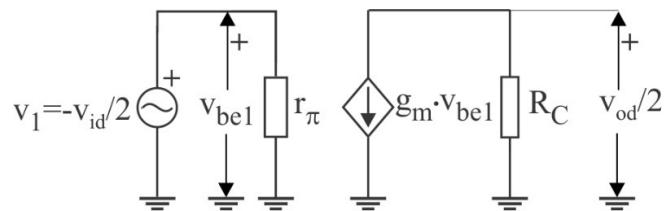
$$v_2 = -v_1 = \frac{v_{id}}{2}$$
