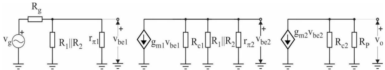
$$A_n = \frac{v_o}{v_g} = \frac{v_o}{v_{be2}} \cdot \frac{v_{be2}}{v_{be1}} \cdot \frac{v_{be1}}{v_g}$$
