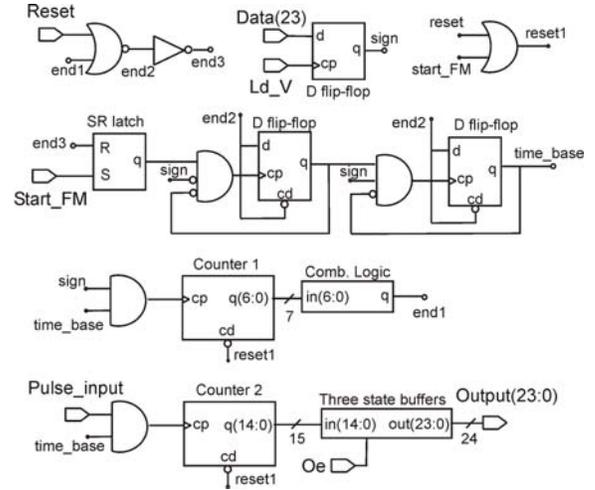
Figure 6. Internal structure of counting circuitry
