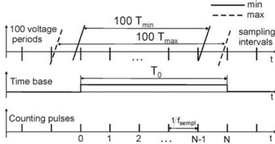
Figure 4. Maximum and minimum durations of 100 power voltage periods relative to sampling intervals
