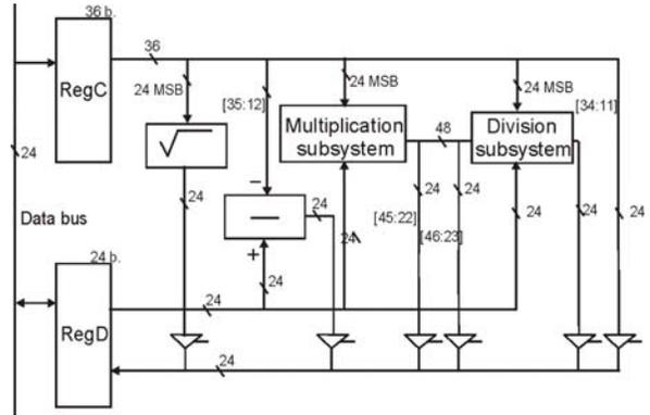
Figure 9. Block of  $I_{eff}$ ,  $V_{eff}$ ,  $P$ ,  $Q$ ,  $S$ ,  $\cos(\phi)$  and Frequency calculation
