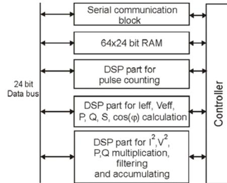
Figure 2. Parts of DSP
