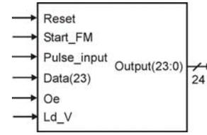
Figure 5. Pulse-counting circuitry interface
