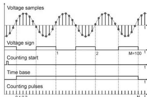
Figure 3. Signals relevant for frequency measurement
