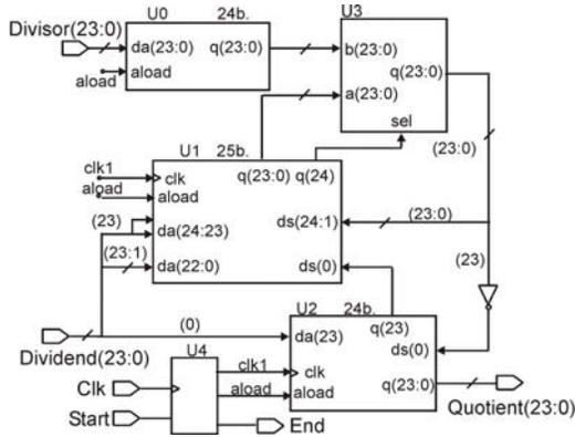
Figure 8. Internal structure of division system
