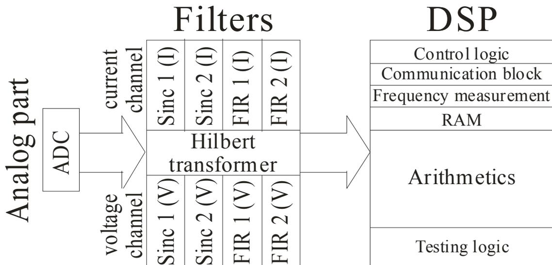
Fig. 1. Architecture of the digital part of the power-meter IC
