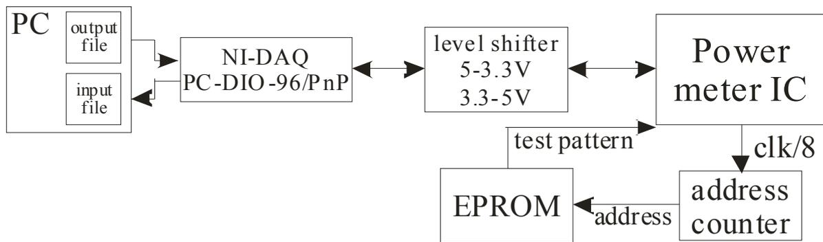
Fig. 3. Set-up for DSP testing
