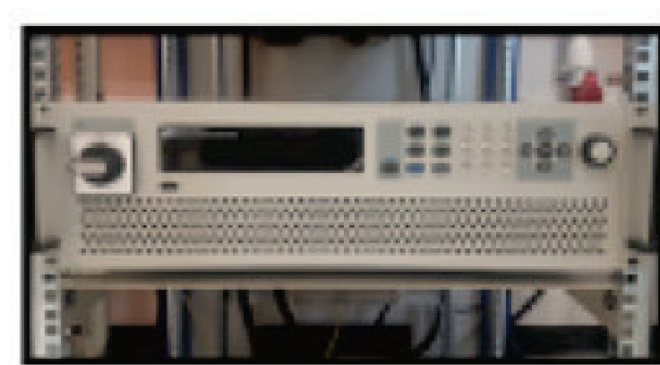
PV panel emulator
