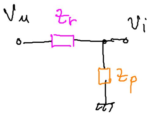
$$H(s) = \frac{v_i}{v_u} = \frac{z_p}{z_p + z_r} = \frac{\frac{R_2}{1 + sC_2R_2}}{\frac{R_2}{1 + sC_2R_2} + R_1 + sL_1}$$
